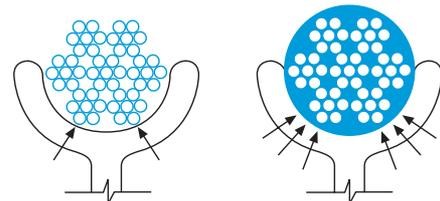
Contact of conventional wire rope with the winding drum and sheaves inevitably leads to high pressure point contact where individual wires meet the contour of the groove. With PIR rope the load is spread and wear on both the rope and drum are minimised.
