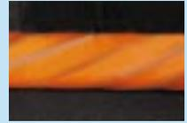
Plastic impregnated ropes have been successfully used on coal and ore unloaders and also in piling operations.
