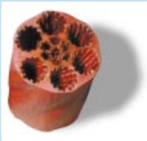
The steel wire rope is impregnated by a special process whereby the individual strand gaps within the rope are filled with a sealing thermoplastic material forming a protective layer between the individual strands and around the core of the rope.
