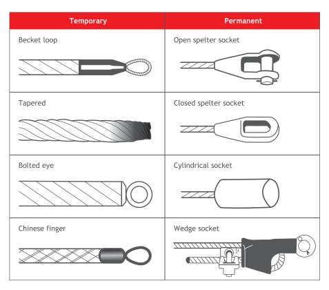
Figure 35 Examples of rope terminations
