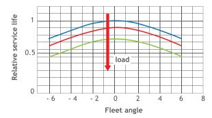
Figure 53 Effect of fleet angle on service life
