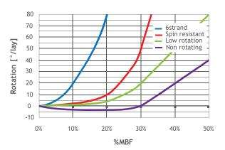
Figure 21 Rotation for different rope constructions
