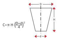
Figure 37 Resin content and cone dimensions
