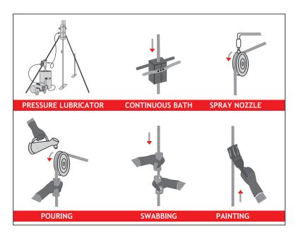
Figure 49 Typical lubrication modes
