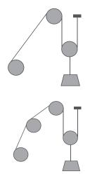
Figure 42 2 Falls with 2 rotating sheaves and with an extra sheave
