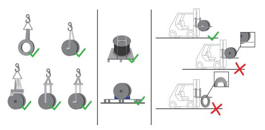
Figure 28 Rope handling recommendations
