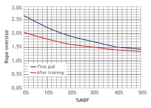
Figure 18 Rope oversize versus load
