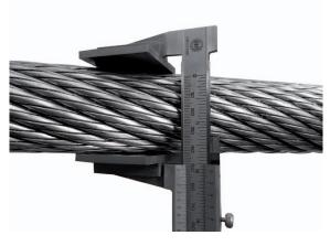
Figure 1 Diameter measurement
