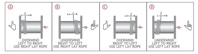
Figure 6 Selection of lay direction
