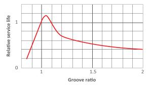
Figure 54 Effect of groove ratio on service life
