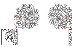
Figure 16 Cushion layer versus plastic impregnated core
