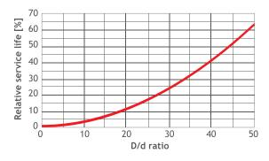
Figure 52 Effect of bending ratio on service life
