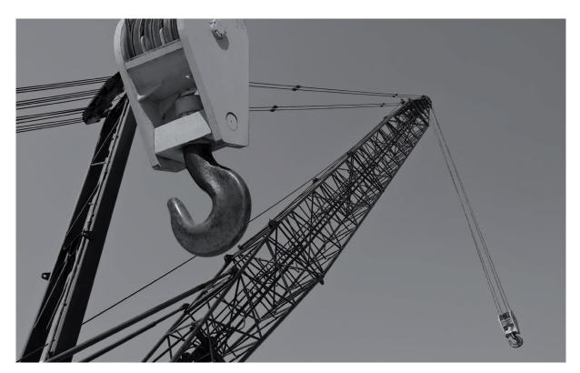
Figure 22 Multiple fall lifting
