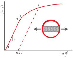
Figure 17 Stress - strain curve for a wire rope
