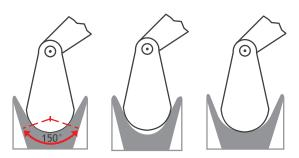
Figure 57 Grooves inspection: correct size, narrow and large groove
