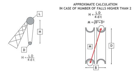
Figure 23 Calculation of maximum lifting height
