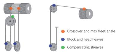
Figure 56 Areas requiring detailed inspection
