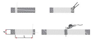
Figure 30 Serving dimensions and configuration
